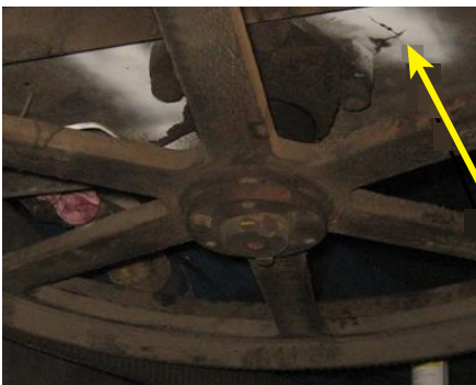
Beam cracked due to repeated shock loads during power up while unit was windmilling.
