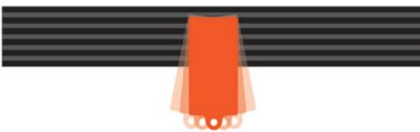
WHEN THE GAUGE ALLOWS LATERAL ROCKING MOTION, THE BELT IS IN NEED OF REPLACEMENT.
