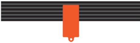
WHEN THE GAUGE REMAINS TIGHTLY SEATED AND RESISTS MOVEMENT, THE BELT HAS SUFFICIENT SERVICE LIFE LEFT.
