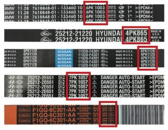
A "PK" number is a worldwide standard metric belt measurement printed on most serpentine belts.
