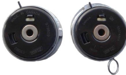
FIG 1: GATES TENSIONER T43143 ON THE LEFT, OE GM TENSIONER ON THE RIGHT; VIEWED FROM THE BACK SIDE.
