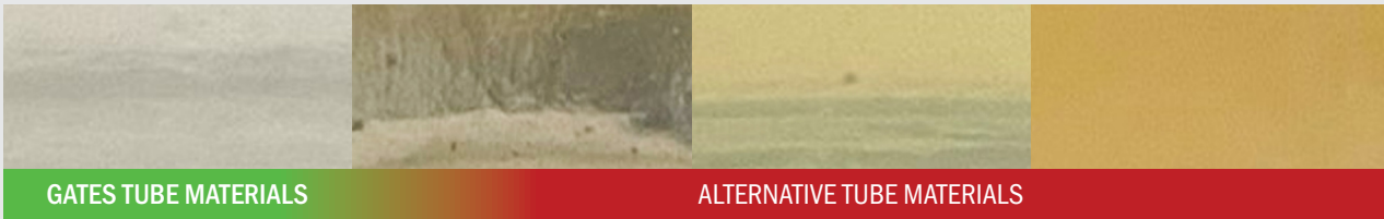
PG25 COOLANT AFTER EXTRACTABLES TESTING WITH VARIOUS DATA CENTER HOSES AT 80°C FOR 600 HOURS
