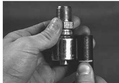
3. Place a visible mark on hose cover at the insertion length shown in the crimp data manual or use MegaCrimp Insertion Tool (7482-1342).
