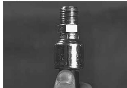
4. Insert coupling into the hose until the mark lines up with the end of the coupling ferrule.
