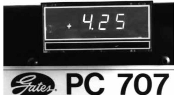
11. Turn knob to a setting below the desired setting. Then turn knob back up to the desired setting. (Digital readout numbers may jump a number, e.g., 5.50 to 5.49 or 5.51. This will not affect crimp diameter of the coupling.)
