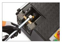
Positioning of cutting ring
