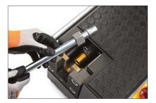
Nut an cutting ring onto tube
