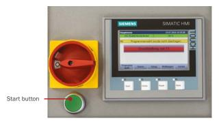
When using a proximity switch the process is started by pushing the tube against assembly socket. Also releasing leads to interruption of process.
