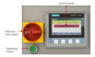
The piston rod is set in motion by pressing the green operating button next to the control panel.
