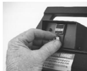
10. Tighten the set screws and replace the plastic cap. Crimper is now calibrated.
