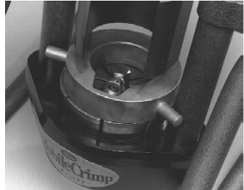
**6. SWING CYLINDER INTO CRIMPING POSITION**
