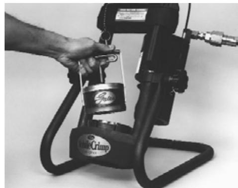
Apply a thin layer of Molykote lube to the top of the die set.
