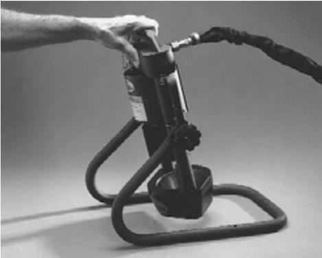
Turn the knob on the controller to a setting of **400**, which allows the ram to extend approximately 1”.
