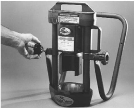
Slide the two halves of the stand together and attach to the crimper at the pivot bolts.
