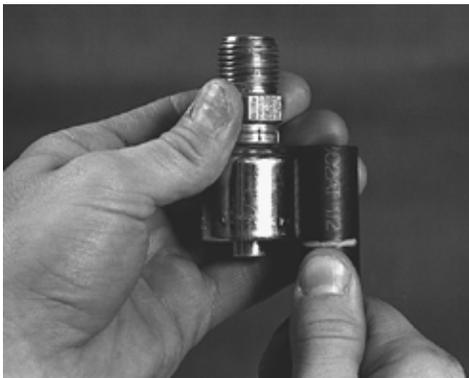
4. Insert coupling into the hose until the mark lines up with the end of the coupling ferrule.
