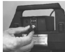
8. Loosen the two set screws in the brass knob 1/4 to 1/2 turn using a .05" Allen wrench.
