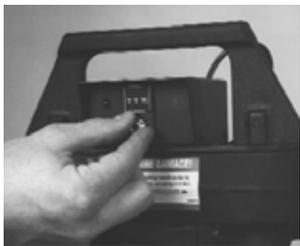
*Note: Rotating the knob on front of switch box clockwise will increase the number; counter clockwise will decrease the number. When changing the setting, always move to a higher number then down to the desired setting. (Ex: To change from 200- 245, move dial up to 300 then down to 245.)*
