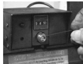
9. Turn the brass knob either clockwise or counter clockwise to get the setting back to 245.
