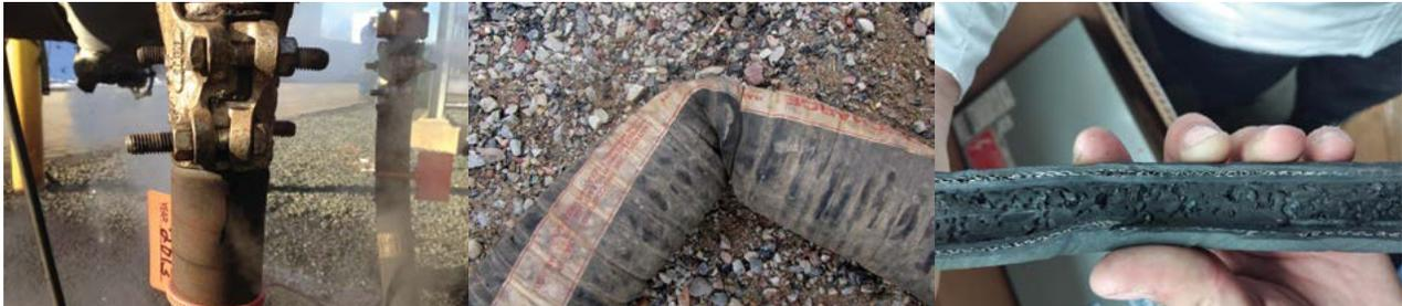
Hose bursts or cracks
