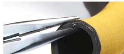
Pinching the staple into the tube wall.
