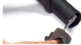
Helix wire being bent into the inner surface of the hose tube.
