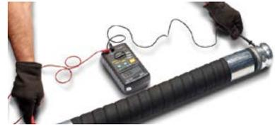
Hose assembly being tested with ohmmeter.
