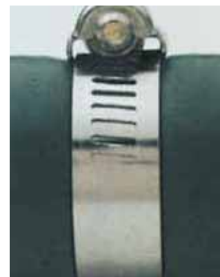
HOSE INSTALLED WITH LINED CLAMP
