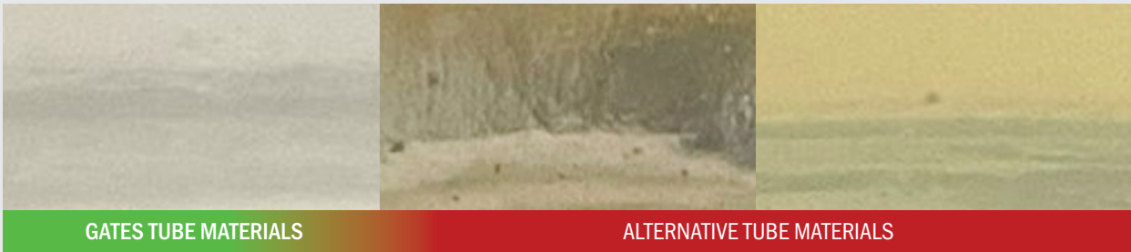
PG25 COOLANT AFTER EXTRACTABLES TESTING WITH VARIOUS DATA CENTER HOSES AT 80°C FOR 600 HOURS
